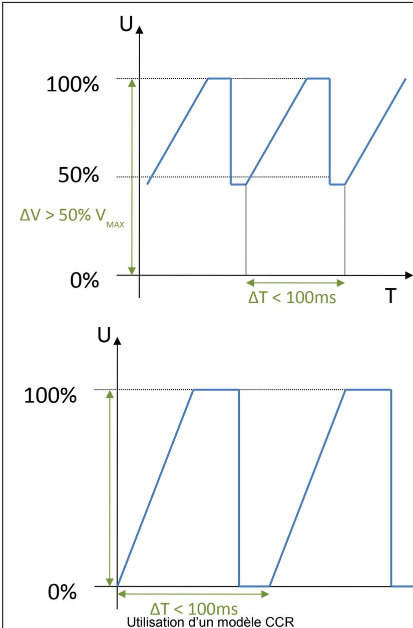
The Capacitor charger (CCR) can be considered as a current generator (Norton model). He's suitable for all applications that need very fast regulation with big voltage amplitudes and repeated charging and discharging (total or more than 50% of the max).
