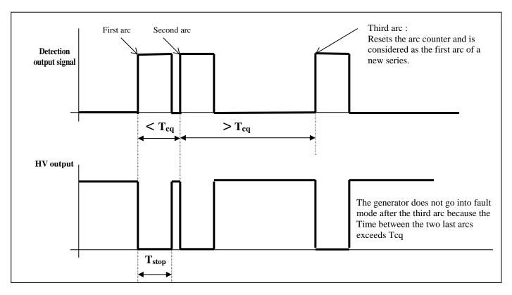
Example 2: User has set the arc counting limit to 3. The third arc occurs a long time after the second arc, and thus resets the arc counter.
