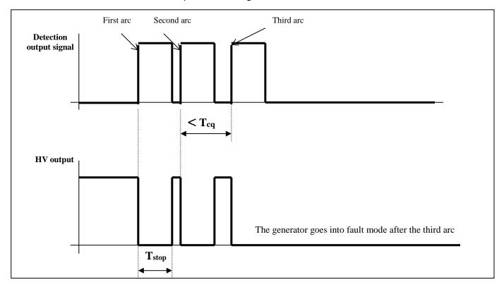
Example 1: User has set the arc counting limit to 3. The generator goes into fault mode after a series of 3 consecutive arcs.
